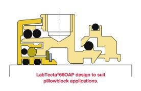
Sealing applications covered with powder or slurry are challenging for any standard bearing seal. The LabTecta®66OAP is specifically designed for this environment ensuring no contamination can enter the seal and compromise its performance.
