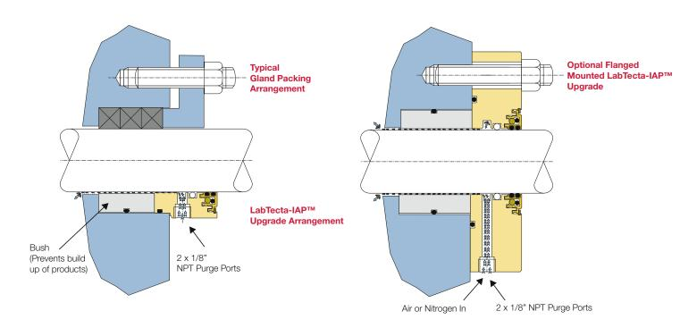
Sealing fan housings is made easy with the LabTecta®66IAP. The positive air purge will contain any emissions or contamination that tries to escape. With no contacting parts during operation, there is no vibration and no maintenance required.
