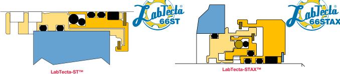
For smaller steam turbines, the LabTecta-ST™ design provides excellent protection in a compact package. For larger steam turbines, the LabTecta-STAX™ provides easy installation with the capability to accommodate large axial shaft movement.
