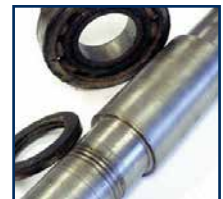
Shaft damage from a labyrinth seal
