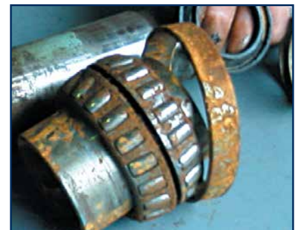
Moisture contaminated bearings
