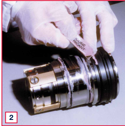
2 Apply grease to the outboard stationary 'O' rings and inboard rotary 'O' rings.
