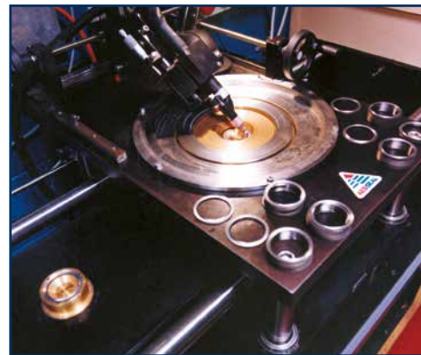
CNC inside diameter bellows welding operation.
