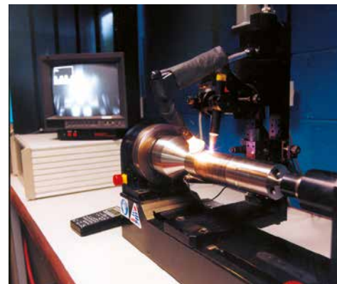
CNC outside diameter bellows welding operation
