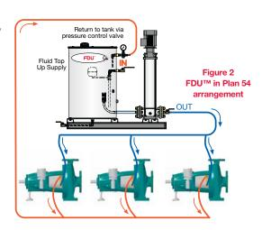
The diagram to the left illustrates how the FDU™ can supply multiple seal support systems. The diagram above illustrates how the FDU™ can supply multiple seals in a closed loop operation.
