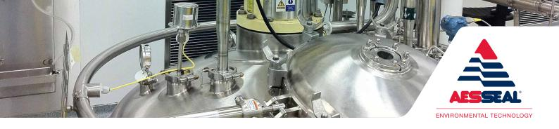
The SW2<sup>TM</sup> connected directly to the plant water line, which became both its fluid and pressure source. The barrier fluid pressure was maintained at 1 bar/15psi above the stuffing box pressure, protecting the seal faces from the harmful process fluid.
