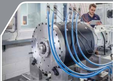
Large diameter dry gas rig
