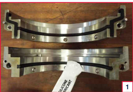
1 Ensure rotary holder gaskets (10) are greased & seated in their grooves along with the shaft o-ring (4) in both halves.
