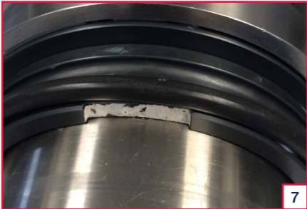
7 Press the rotary face (8) and 'O' ring (9) sub-assembly into the rotary holder (6), ensure the slot in the face aligns with the pin(s). Remove the rotary holder spacer shims (19). Equally tighten rotary cap head screws (7) (SEE TABLE 1 FOR TORQUE SETTINGS) and clean the face with aerosol non-CFC solvent cleaner.
