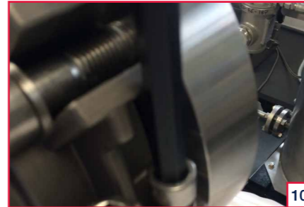
10 Fit the top gland half (1) and lightly tighten the M12 gland caphead bolts (2).
