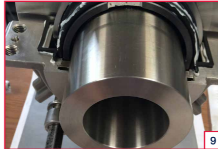
9 Lubricate gland 'U' seals (17) and fit gland half (1) (use stuffing box bolts to support gland as necessary). Ensure that gland pin (15) is aligned with the slot in the stationary face shown in white.
