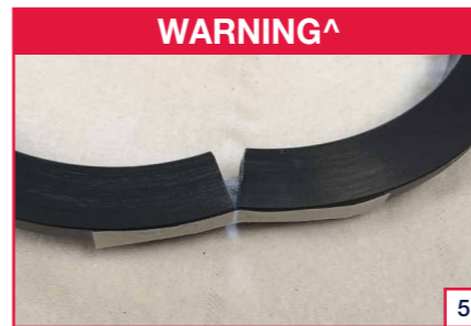
5 Add supplied "steri-strip"(20) to face (8^A) edge, ensure it does not rest on the running surface. Note the position of the anti rotation slot.
