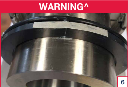
6 Open the rotary face over the shaft allowing the tape to hold the seal face in place. Locate the 'O' ring (9) around the seal face. Repeat step 4 for the stationary 'O' ring (12) then open the stationary face (11^A) over the shaft allowing the tape to hold the face in place whilst locating the stationary 'O' ring (12) around the stationary face. Remove the face tape (20) from both the rotary and stationary faces.
