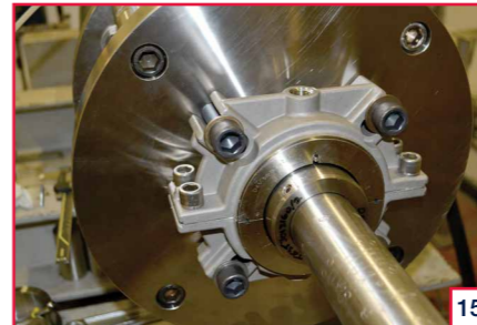
15 Connect flush if required and vent seal prior to start up.
