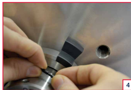
4 Fit split rotary 'O' ring (9) over shaft and join using adhesive supplied and lubricate the 'O' ring.
