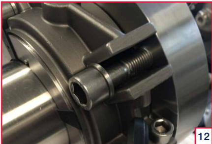
12 Fully tighten the gland cap head screws (SEE TABLE 2 FOR TORQUE SETTINGS)
