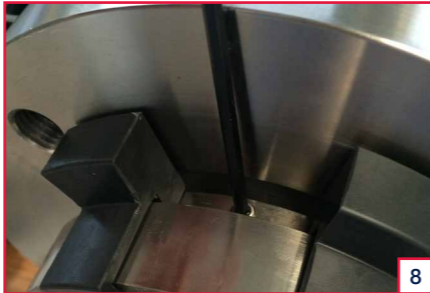
8 Equally tighten the M6 drive screws (5) to 5Nm (3.5lbf-ft) remove setting clips.
