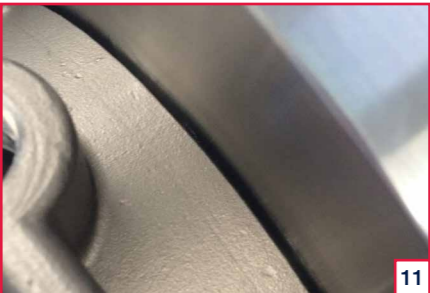
11 Fit upper stuffing box bolts and equally tighten until gasket contacts stuffing box face.
