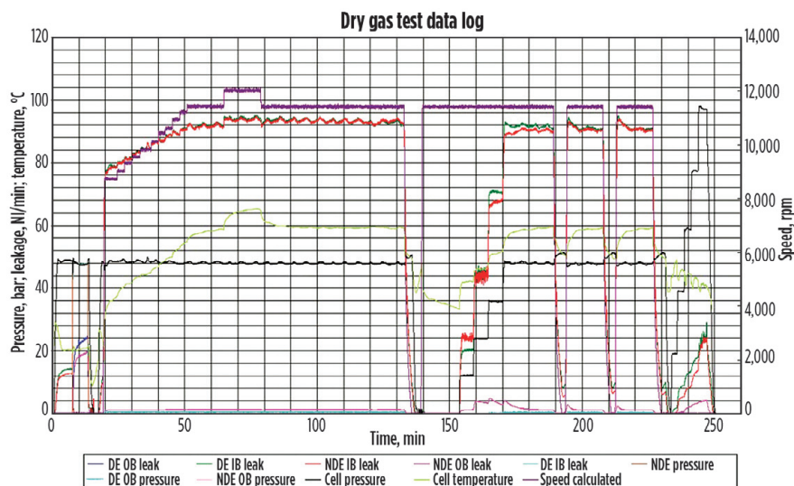
FIG. 5. A typical graph relating to the logged data taken during a comprehensive DGS dynamic test, where pressure and speed are varied to suit future operating conditions. Source: AESSEAL plc.
