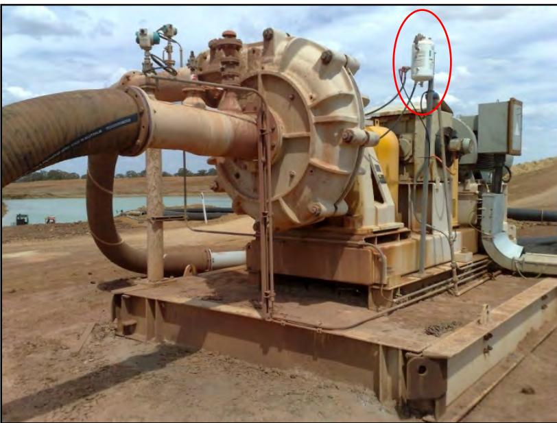
Figure 12. Same Warman slurry pump as above, AFTER installation of double mechanical seal and tank system (in circle).
