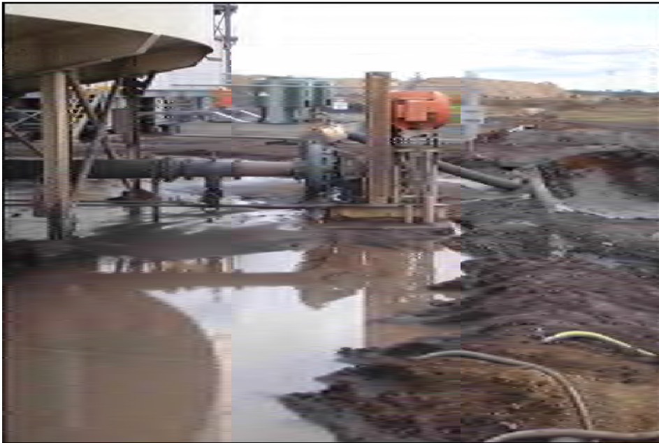
Figure 2. Typical mining slurry pump with packing gland water can create a safety hazard and waste water.
