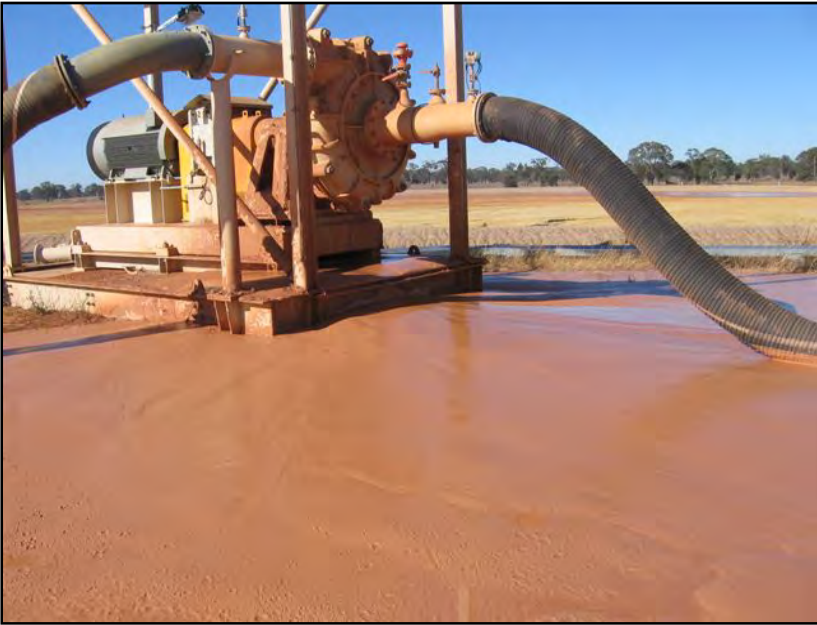
Figure 11. Warman GAH slurry pump with leaking packing gland water, BEFORE installation of mechanical seals.
