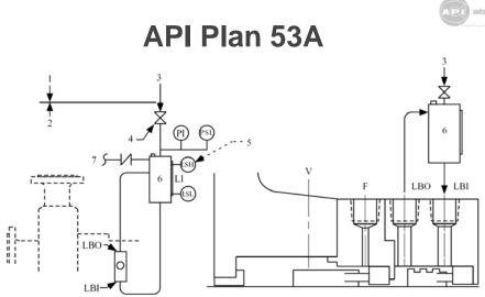
Pressurised external barrier fluid reservoir supplying clean fluid to the seal chamber. Circulation is by an internal pumping ring. Reservoir pressure is greater than the process pressure being sealed.
