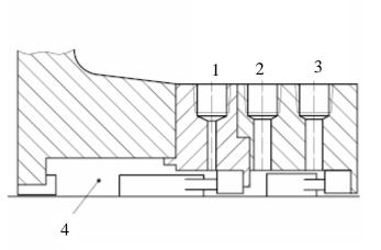
Dual Seal 1 Flush 2 Barrier Out 3 Barrier In 4 Seal Chamber
