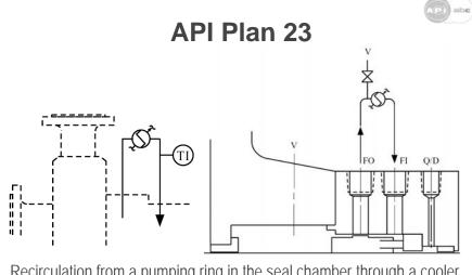
Recirculation from a pumping ring in the seal chamber through a cooler and back into the seal chamber.
