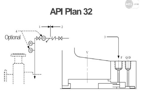
Flush is injected into the seal chamber from an external source.
